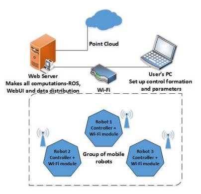
Fig 3.1. Control system for centralized structure of mobile robots
