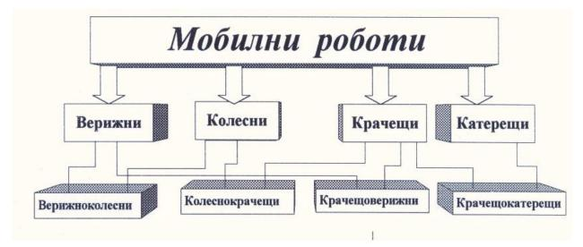
Fig. 1.1. Classification of mobile robots
